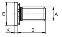
Head diameter E = 10.0 Head height K +/-0.02 = 1.50 Hole diameter +0.1 = 6 Length B +/-0.4 = 34 Male thread A = M6 Min distance to edge = 11.5 Tightening (N m) = 10.0
